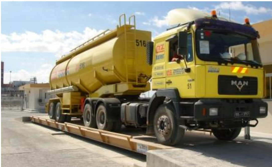
Eurodeck weighbridge from Weightron Bilanciai at the Gabes LPG terminal
