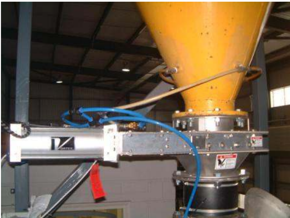
Vortex Roller Gate valve installed beneath a powder hopper
