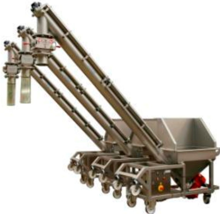
The three inclined Van Beek screw conveyors delivered to KoninklijkeVerkade
