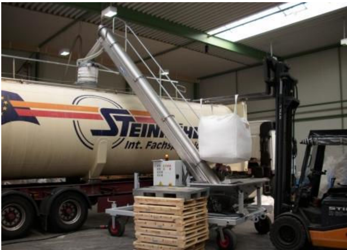
The Van Beek Dino loads material from bulk bags and sacks into a Steinkühler tanker
