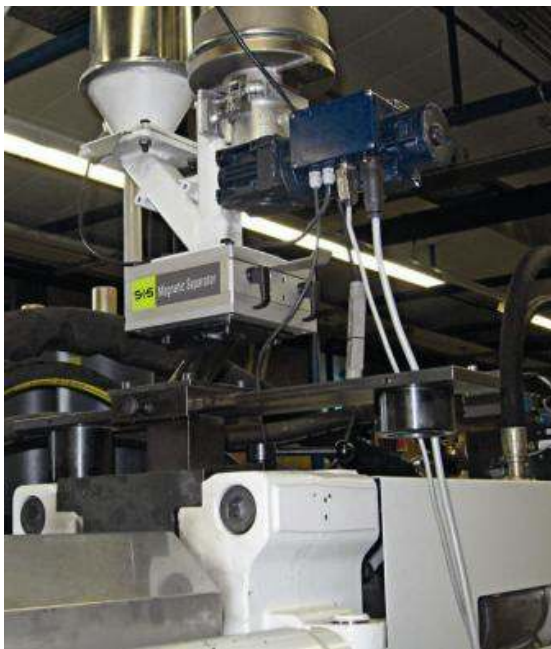
S+S's SAFEMAG installed (left) directly below the metering outlet and (above) units awaiting despatch
