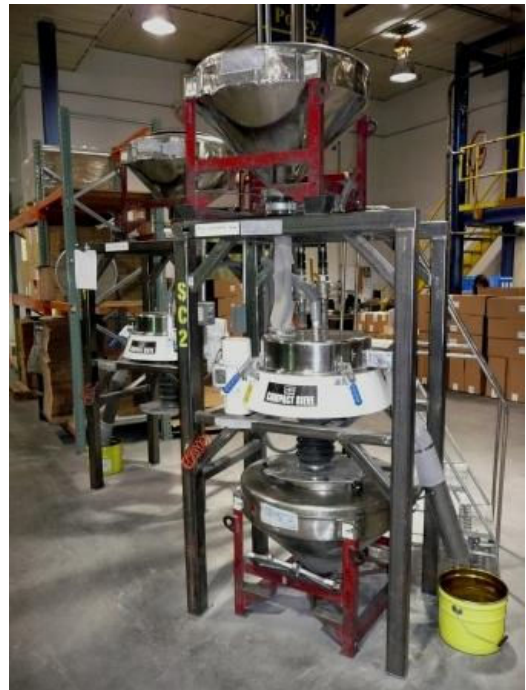
Stainless steel Russell Compact Sieve and (right) a Compact 600 operating in a coatings plant
