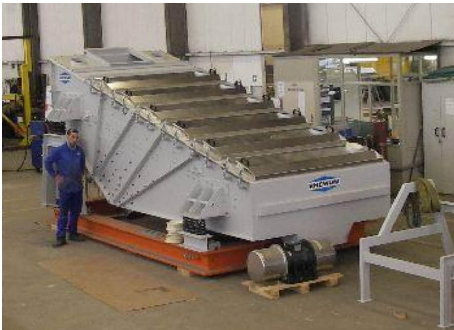
Rhewum RIUS screen fitted with food-grade wear linings for processing rape seed
