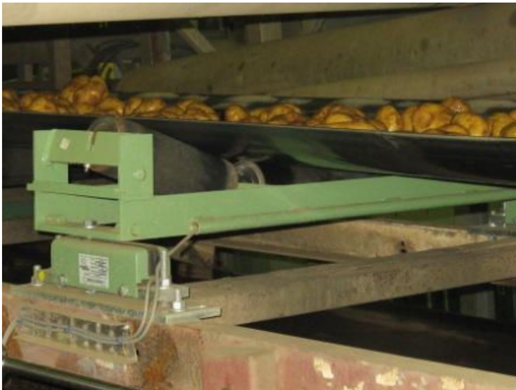
Precia-Molen FX belt scale measures potato intake at McCain Foods
