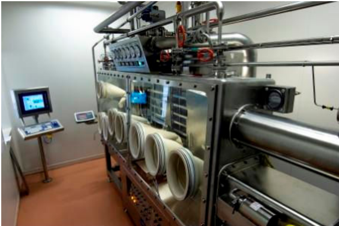
Cake-stand tray drier with PSL high-containment isolator
