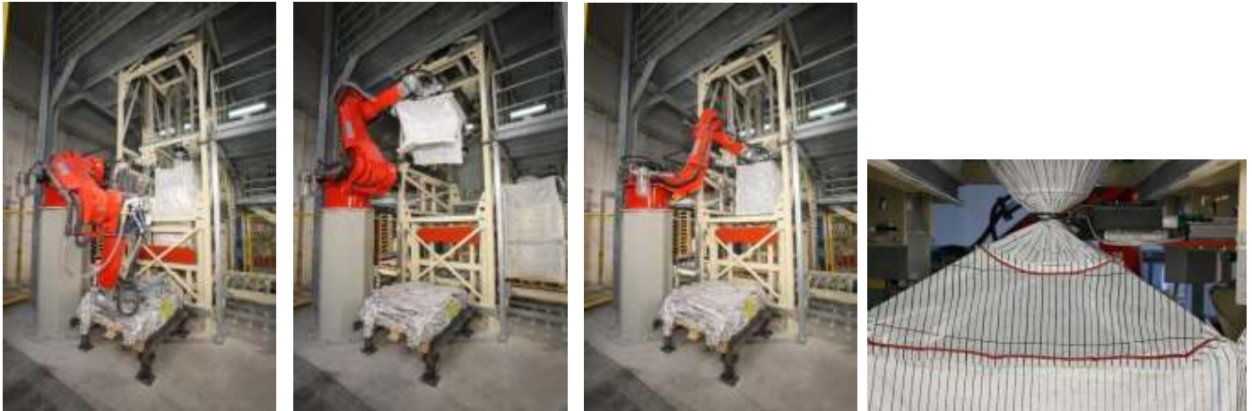
Nordenia/Reis fully automatic 4-loop bag filling system, showing (from the left): the robot picks up an empty FIBC, brings it to the filling rig, connects filling spout and attaches loops, then ties off the spout after filling
