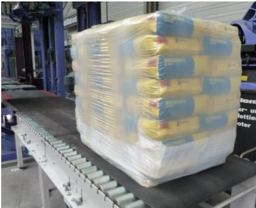
Palletless stretch-package unit comprising 60 x 25kg FFS bags containing cement
