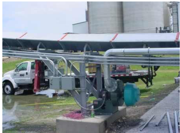
The Martin Engineering air-supported conveyor at Vulcan Materials and (right) the plenum is pressurised by means of a centrifugal fan
