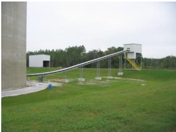
The Martin Engineering air-supported conveyor at Vulcan Materials and (right) the plenum is pressurised by means of a centrifugal fan
