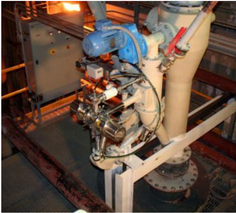
Malvern Insitec fineness analyser installed on a cement line
