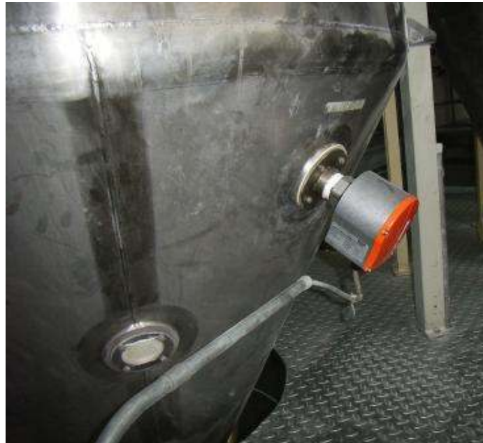
MBA 200 rotating-paddle indicator and (right) installed on a Nordmilch milk powder vessel
