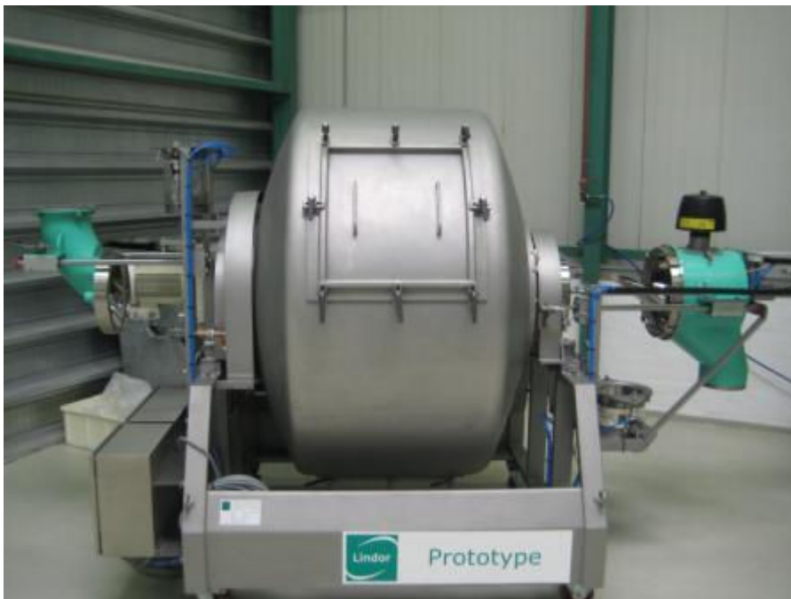
Prototype of new Lindor easy-clean mixer featuring demountable inlet and outlet
