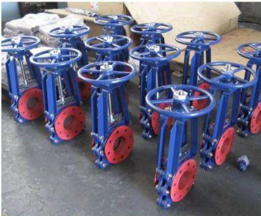
Knife gate valves awaiting despatch; note the Linatex premium rubber linings in their trademark red
