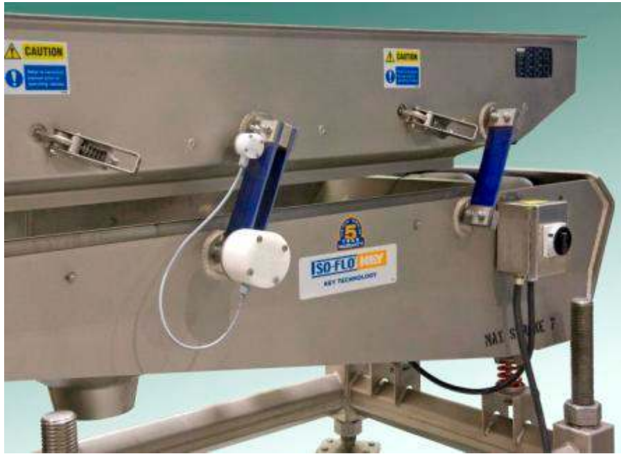
Key Technology's SmartArm fitted to an Iso-Flo conveyor
