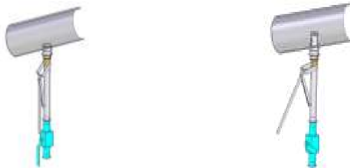
Kersting InlineTasty sampler installed on a pneumatic conveying line, closed (left) & engaged
