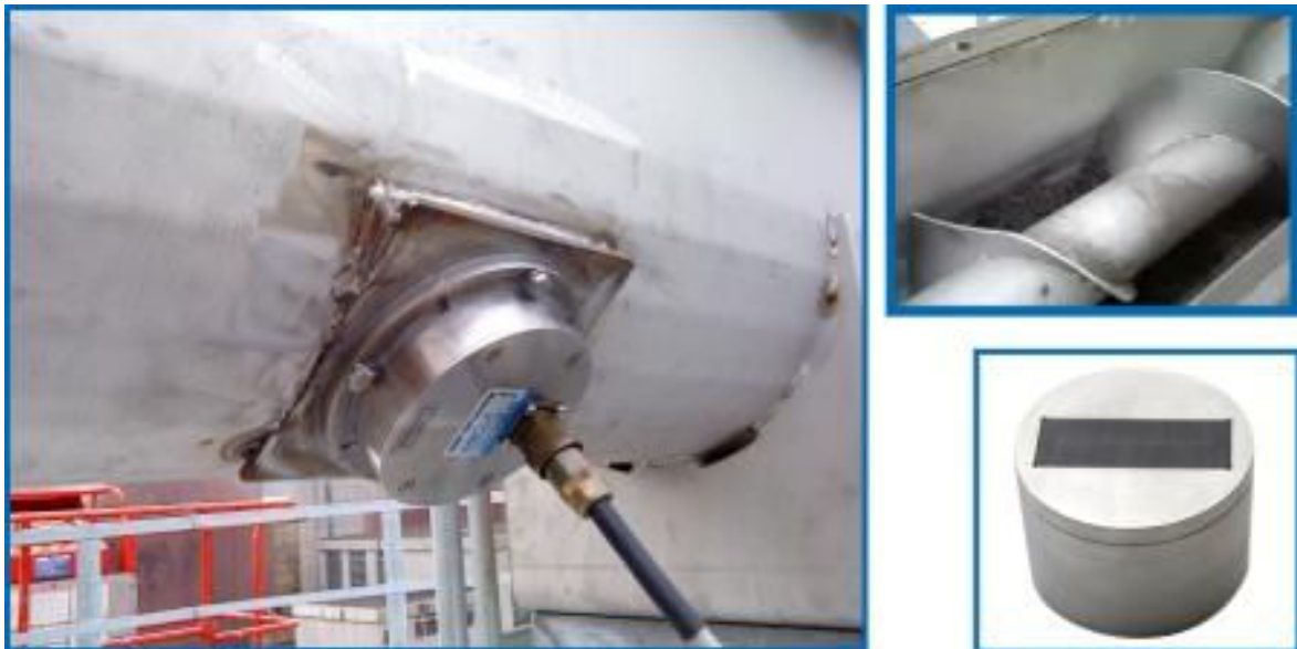
The new moisture probe mounted on the casing of a screw conveyor
