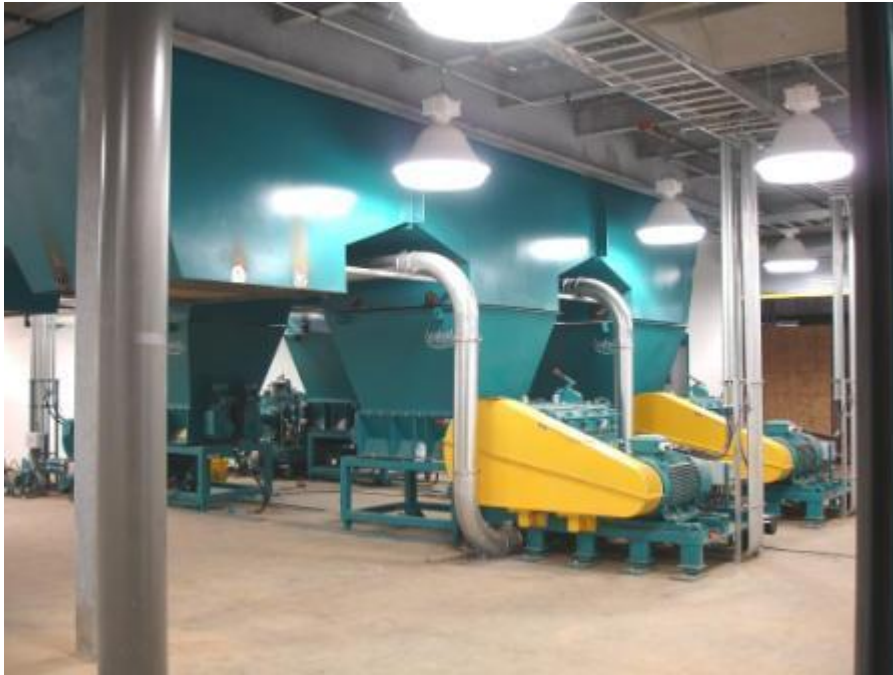
Herbold SB 60/100 granulator (above) and schematic showing forced-feeding mechanism (below)
