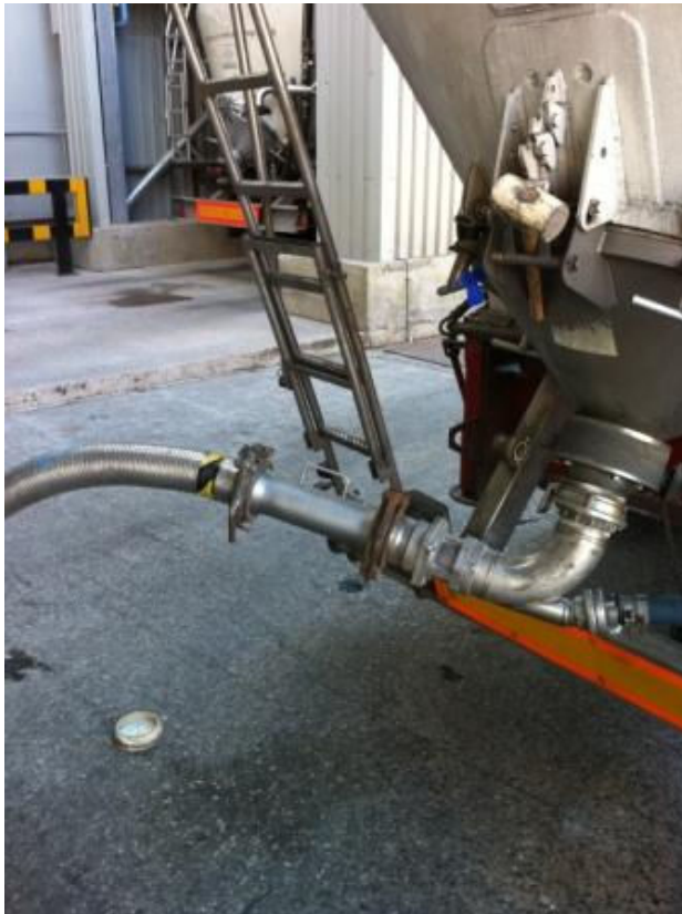
A Greenwood Magnetics Tanker Magnet fitted to a tanker line blowing flour
