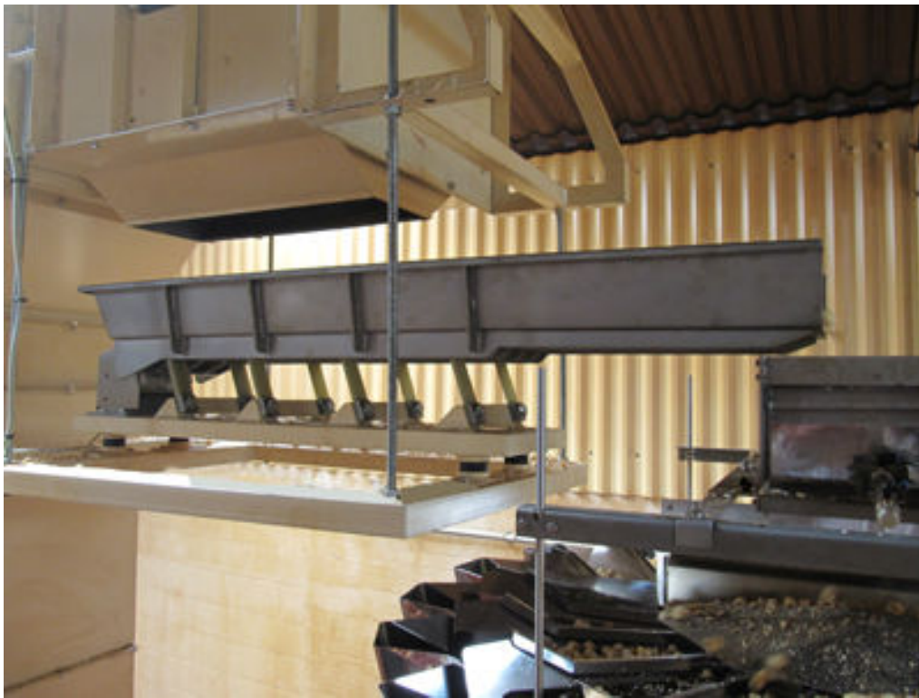
Installation from Gough Engineering for handling popcorn
