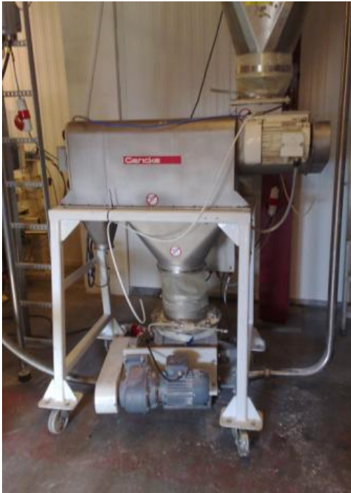
Gericke CSM-722 sifter carrying out trials with animal proteins
