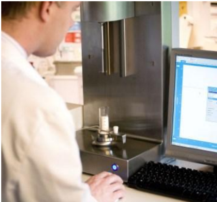
FT4 powder rheometer from Freeman Technology
