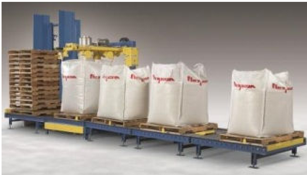
A 15-pallet dispenser releases the bottom-most pallet to roll beneath the cantilevered fill head
