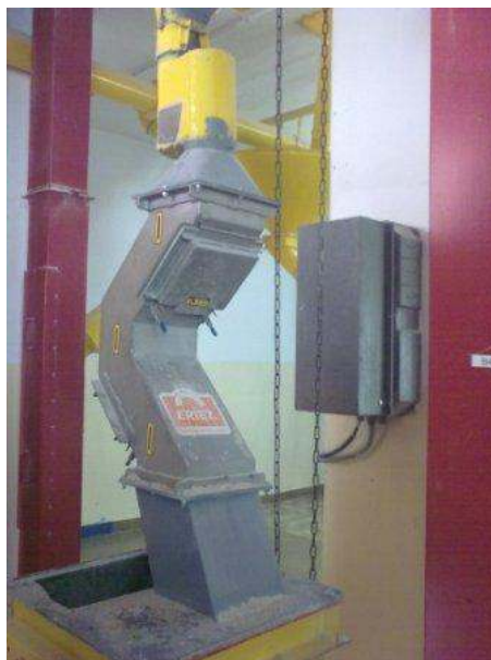
Eriez magnetic hump separator at Granexport showing (right) how it captures ferrous contaminants
