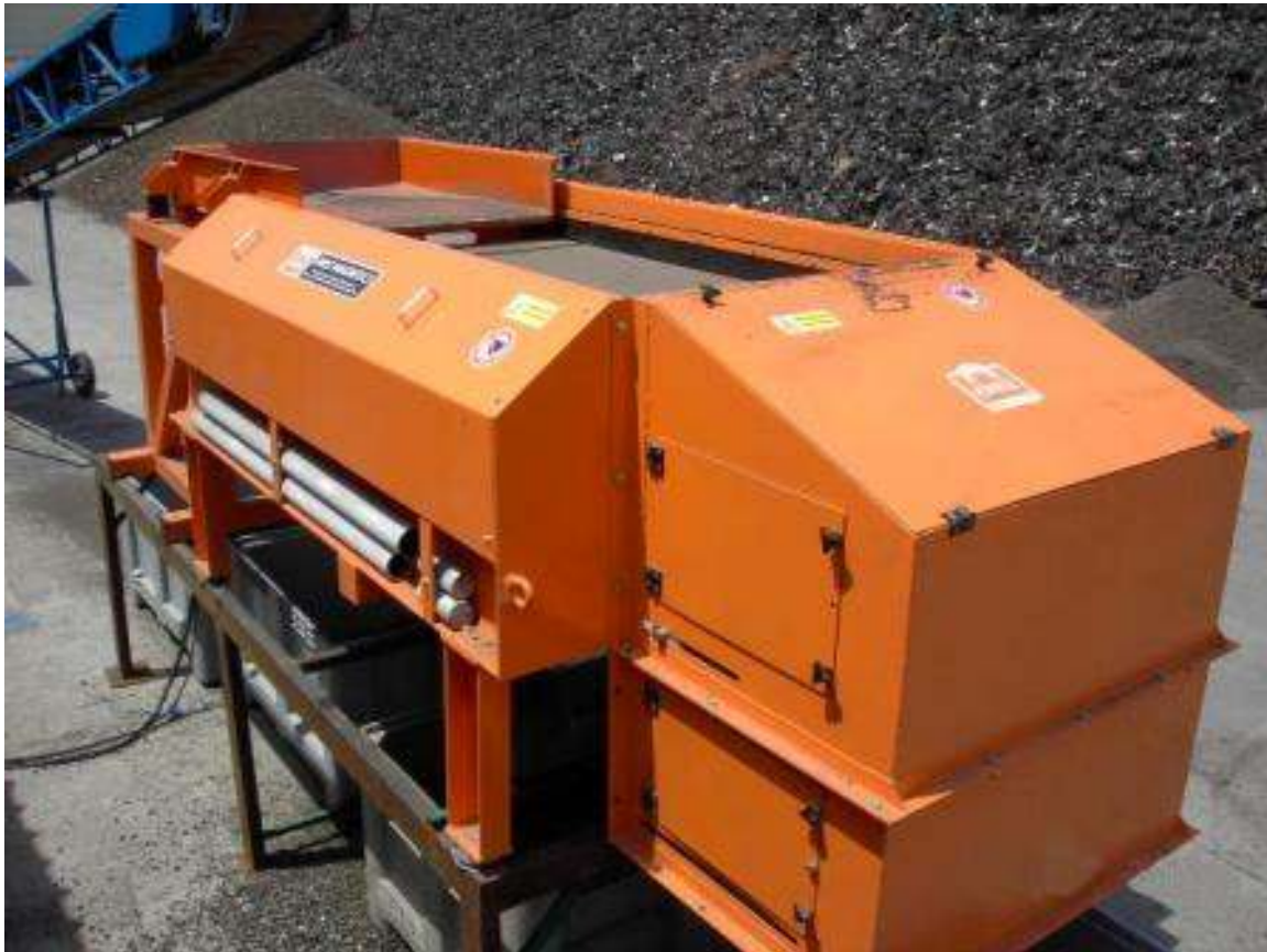
RevX-E eddy current separator from Eriez
