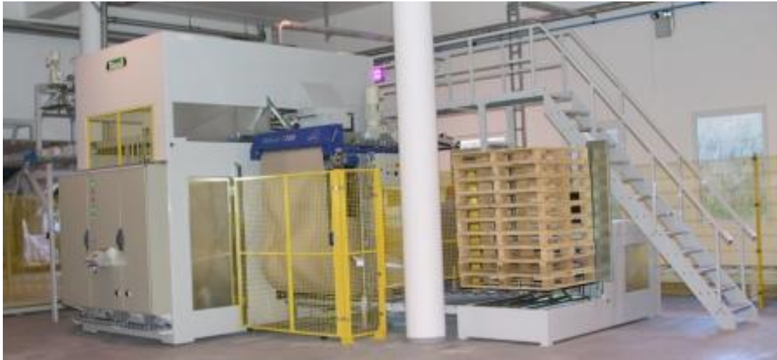
One of Ehcolo's new bag palletisers fitted with servo controls
