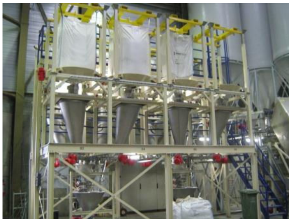
Dinnissen's direct infeed system from bulk bags and (right) detail of the dosing/pneumatic transfer arrangement
