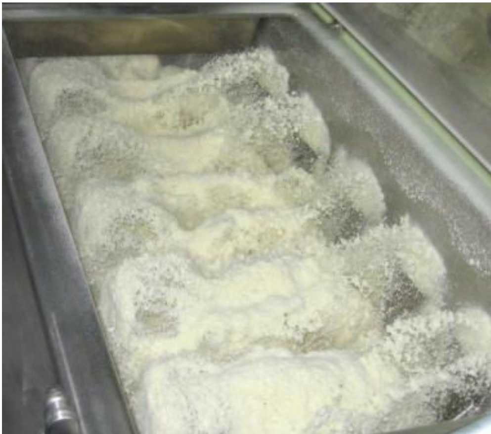
A Pegasus mixer carries out synchronous mixing, spray-coating and drying of fragile ingredients
