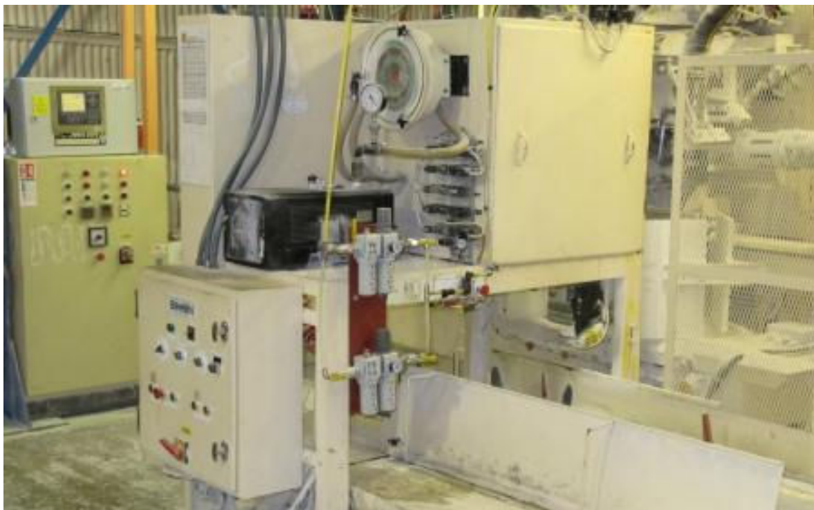
A Richard Simon automatic bag placer has been upgraded by Chronos BTH engineers at the Langley facility of Smiths Flour Mills
