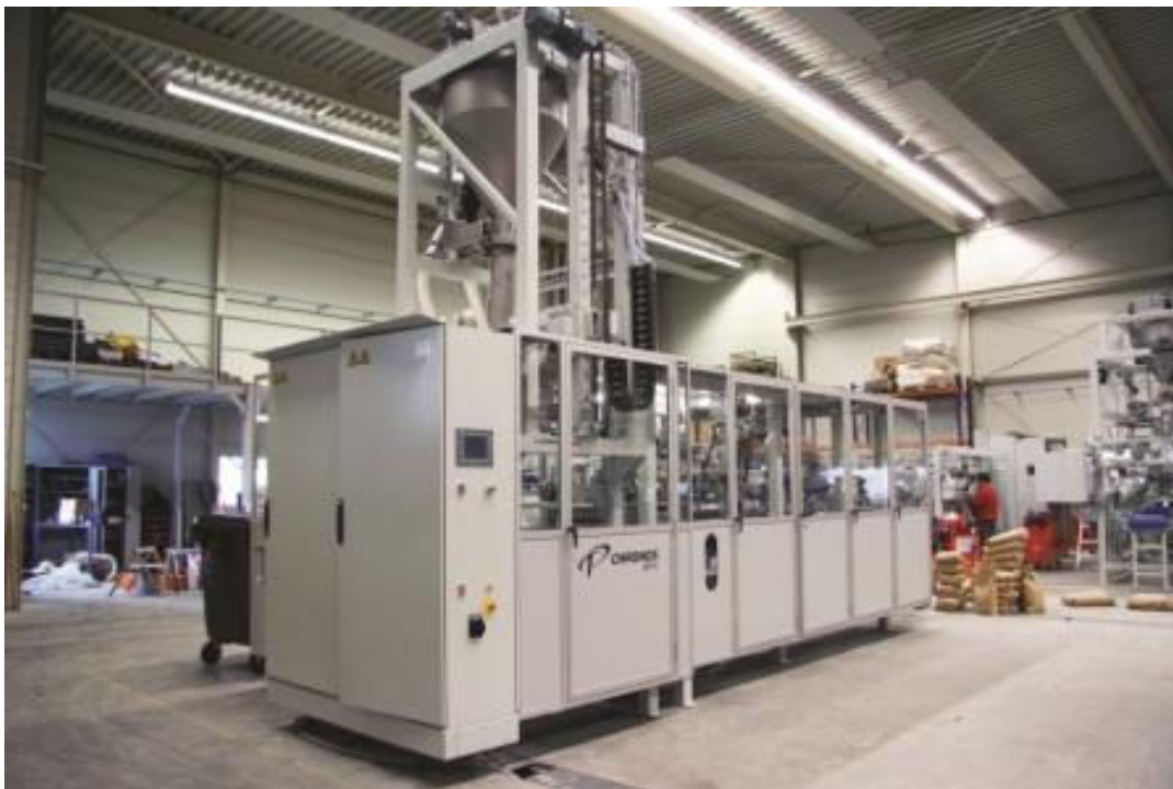
Chronos BTH OML-1030 BF single spout bagging system; dual spout and triple spout versions are also being supplied to Weston Milling
