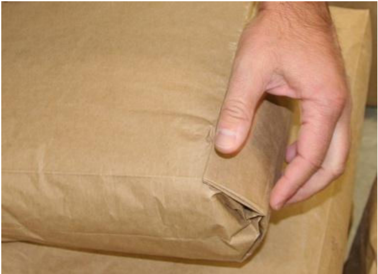
The squared finish of Chronos BTH's BlockTop bag closing method
