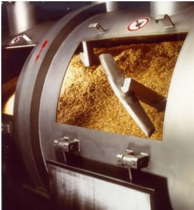
AVA-Huep mixer with blades specially designed for dry spice blending
