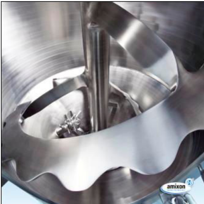
Mixing element from amixon's latest generation of vertical mixers
