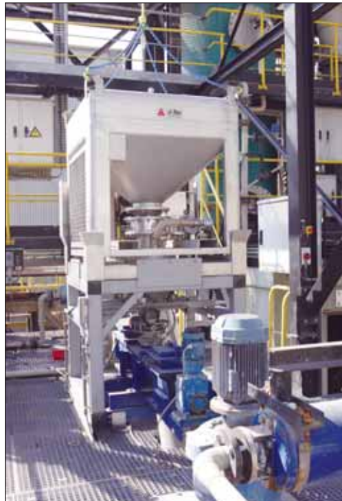
Novel J-Tec powder dosing system at Umicore Oxyde, Belgium, using stainless steel containers.
