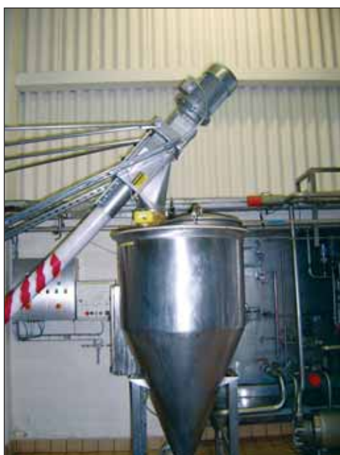
Raw material is transferred from the receiving hopper and gravity fed into the mixer via the transition discharge adapter of the flexible screw conveyor.
