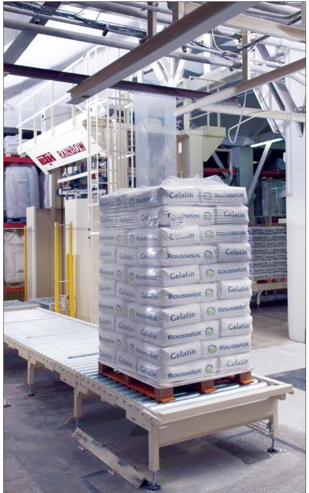
Palletised bags protected by a waterproof and dustproof polythene covering after passing through a BTH Rainbow stretchhood machine.
