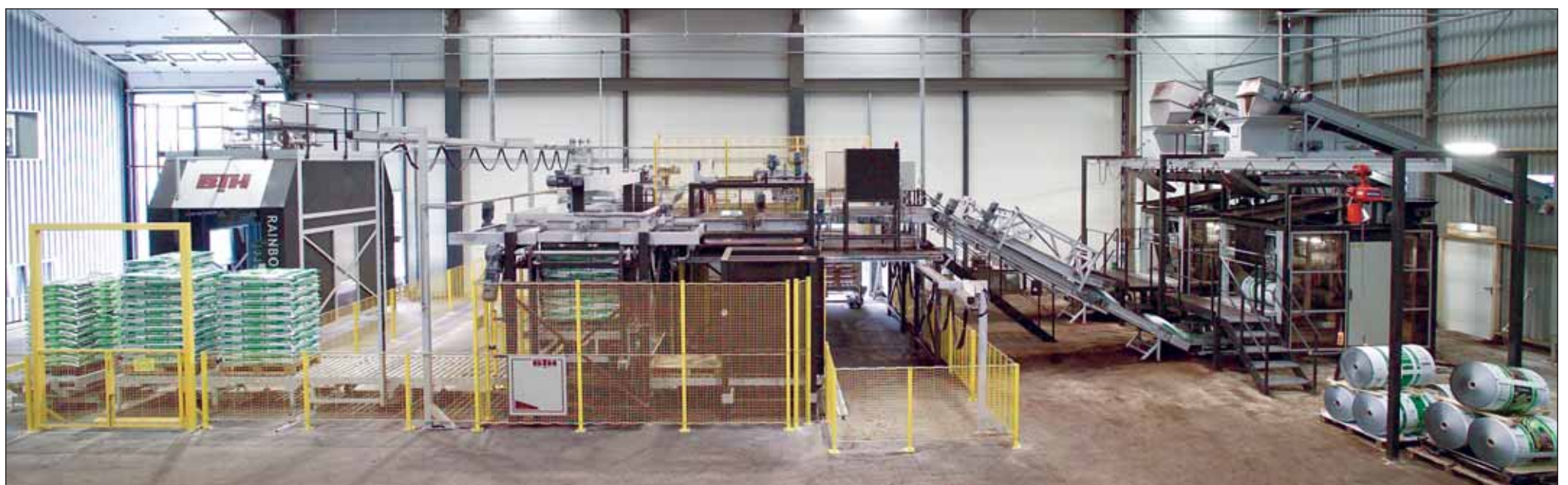
Two fully automatic flat foil bagging lines for potting compost at Dutch garden centre specialist Naturado Bodemvoeding, showing BTH bag fillers, palletisers and a Rainbow stretchhooder; for this type of application very high capacities are normally required.
