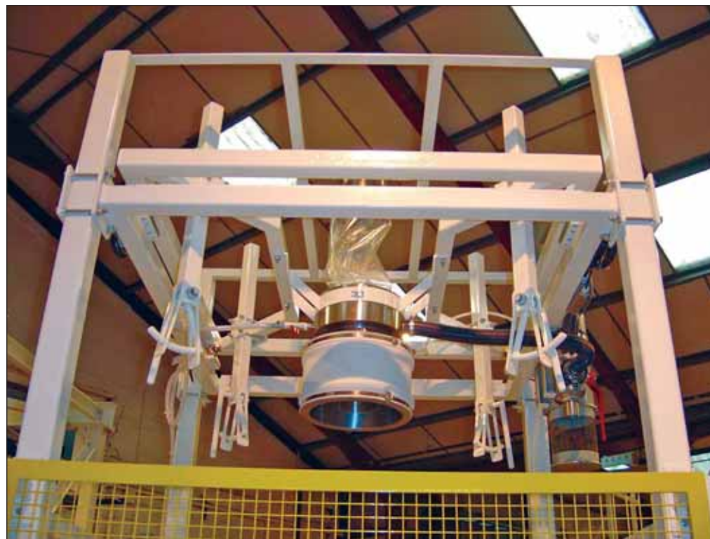
Close-up of the Spiroflow inflatable seal on the filling head which is mounted on the weighing frame.
