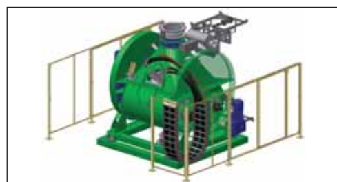
F-RM rotating twin-shaft paddle batch mixer from Forberg International showing loading (left) and discharge positions.
