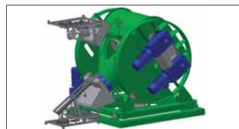
F-RM rotating twin-shaft paddle batch mixer from Forberg International showing loading (left) and discharge positions.
