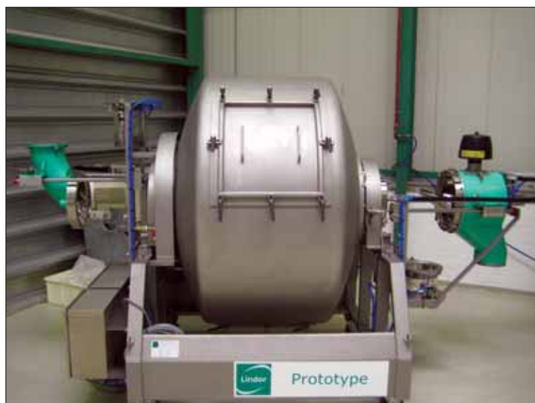
Specialising in manufacturing mixers which are internationally recognised for their gentle handling characteristics, Lindor of the Netherlands has developed a prototype machine (pictured) which features a fully demountable inlet and outlet for quick and easy cleaning for ultra-hygienic applications. This and other recent mixer innovations are described in the feature on p11.
