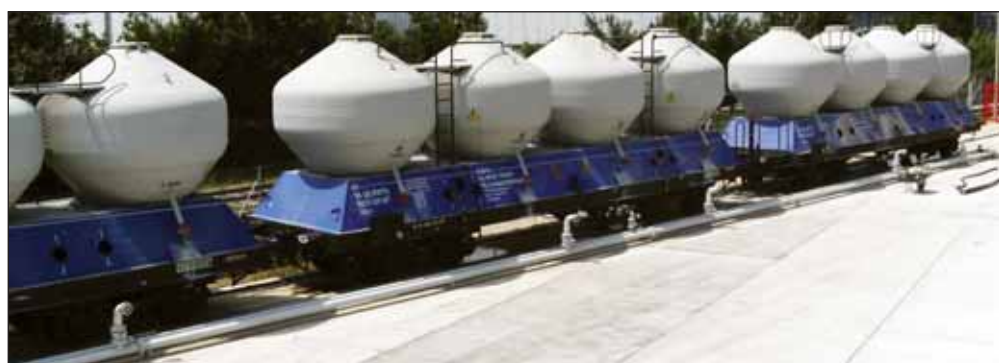
Last year Gericke commissioned a newly developed pneuwork® system at Transportbeton, Austria, for discharging cement from rail tankcars to silo storage.
