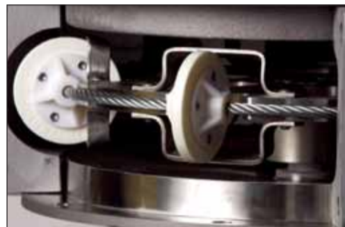
Floveyor's new polymer-coated rope assembly (PCPU).
