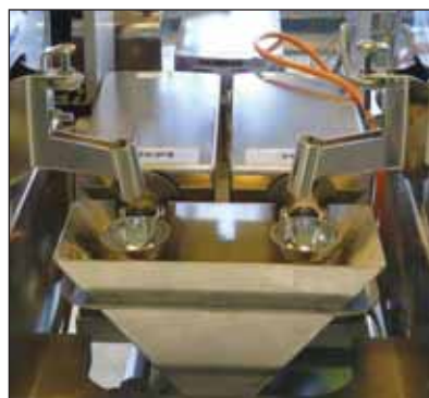
Part of SST's Fine Dosing installation for alumina powder.
