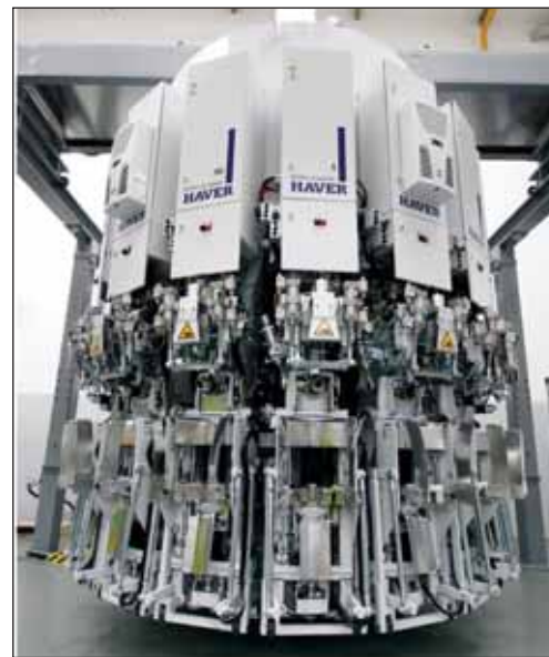
16-spout Haver Roto Classic which is currently being installed at an Indian cement plant.
