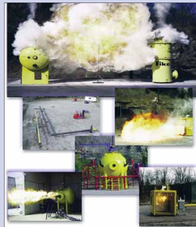
Fike's US full-scale explosion test site allows a wide range of potentially dangerous trials including flame propagation and isolation, explosion suppression and explosion venting to be carried out under safe conditions.
