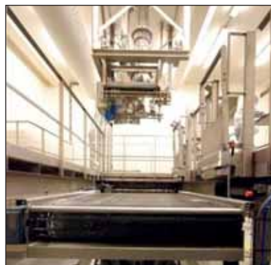
Ultra-hygienic Delaere filling rig for loading lactose into bulk bags at Friesland Foods and (right) mobile polymer filling system in Germany with integral Pelletron DeDuster.
