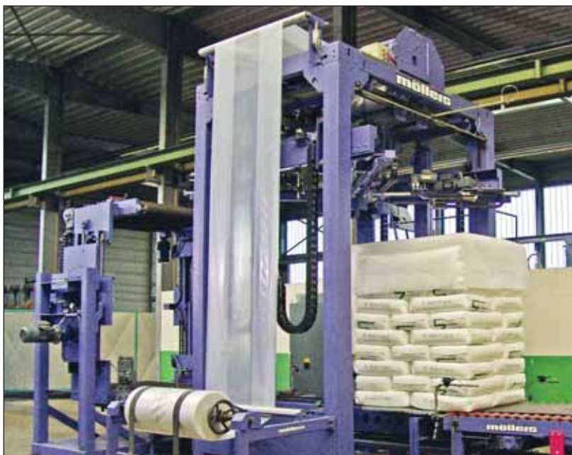
An inner hood of ultra-stretch PE film is drawn down over a bag stack, after which the load is turned through 180 degrees and the reverse (outer) hood is applied in the same way.
