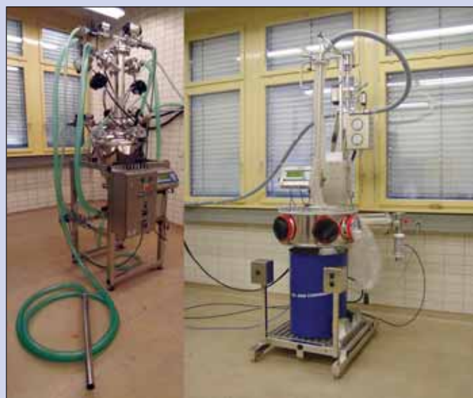
Test equipment at Dietrich Engineering Consultants' Ecublens/Lausanne plant includes a batch mixer (left) and Drum Containment System (DCS) for safe transfer of highly toxic powders.
