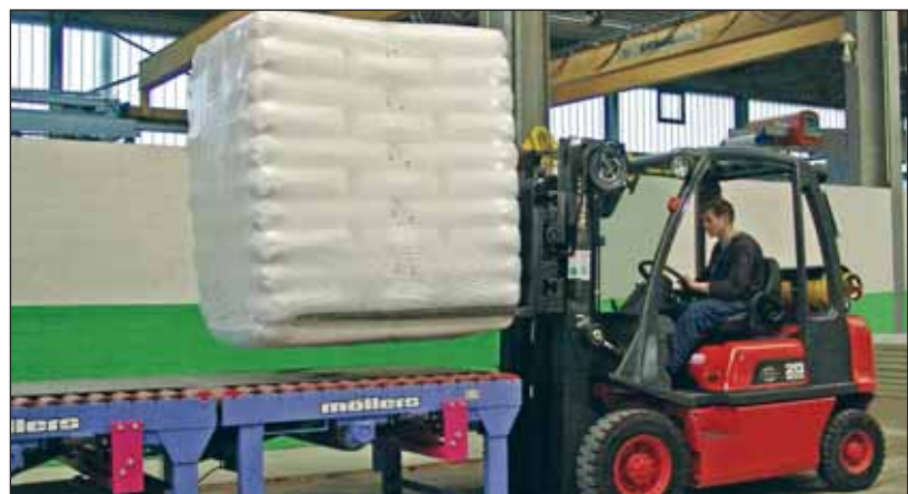
The Möllers pallet-less load is entirely watertight and can be easily handled by forklift.
