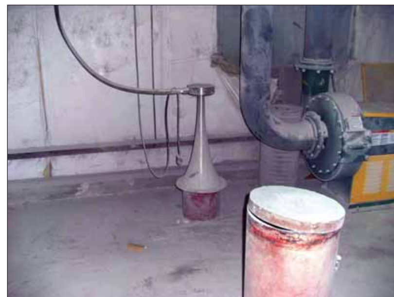
Problems of potassium nitrate hang-up on Ferro Corp's silo sidewalls have been solved with this Primasonics PAS-230 acoustic cleaner.
