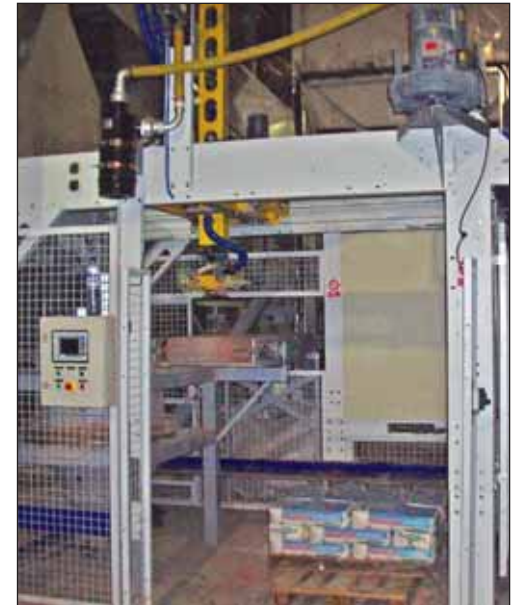
TMI's automatic de-palletiser and bag emptier shares many design features of Robosac P4 gantry palletiser.
