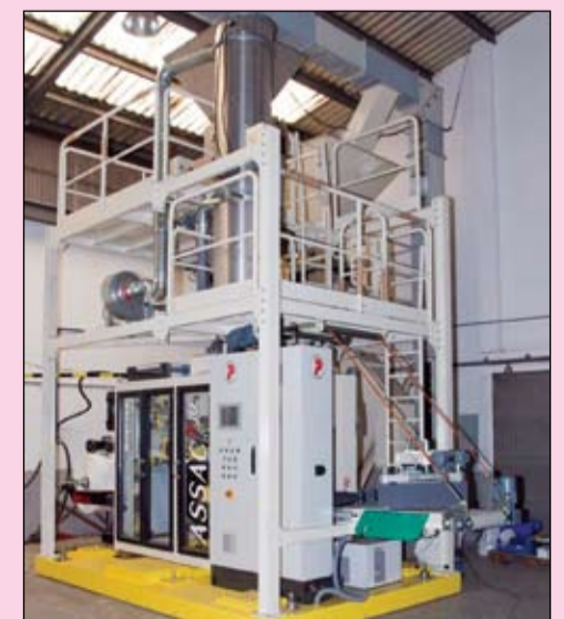
A Payper ASSAC M10 FFS bagging system is among the items of equipment available for trials at the company's test plant.
