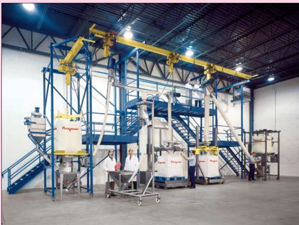
Flexicon test laboratories are divided between equipment that transports, receives or discharges material by means of mechanical conveyors or gravity (pictured), and equipment that transports, receives or discharges through pneumatic conveying lines.
