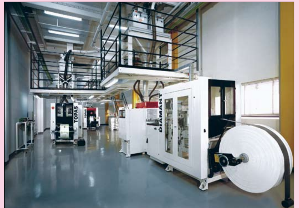
The Lengerich FFS (form-fill-seal) bagging test plant of Windmüller & Hölscher.
