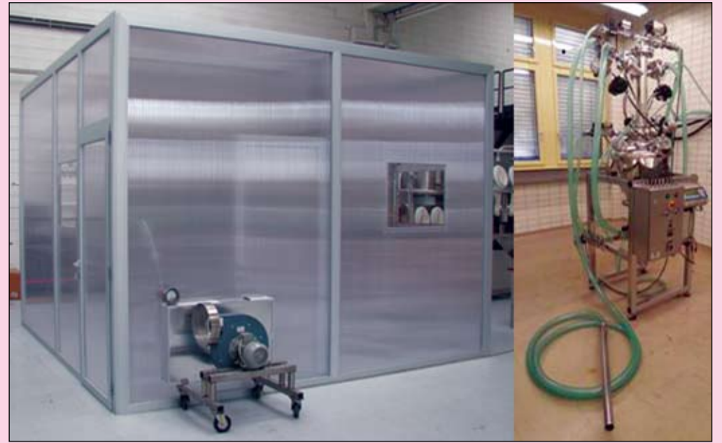
Batchmixer test equipment for powder blending at the Dec Group test plant in Ecublens, Switzerland, and (left) SMEPAC-compliant cabin for containment testing.
