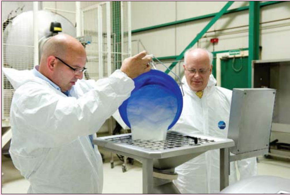
A product formulation being loaded into one of the five different Lindor mixers available for customer trials at the company's Dordrecht facility; here information about mixing effects and final properties of the mixed product can be calibrated.
