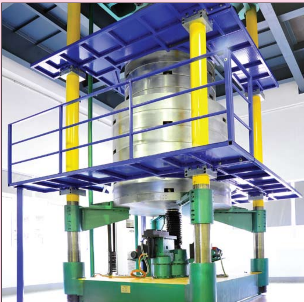
Mettler Toledo test device with 50t direct load capacity for compression weigh modules. A lever test device for 100t is available too.
