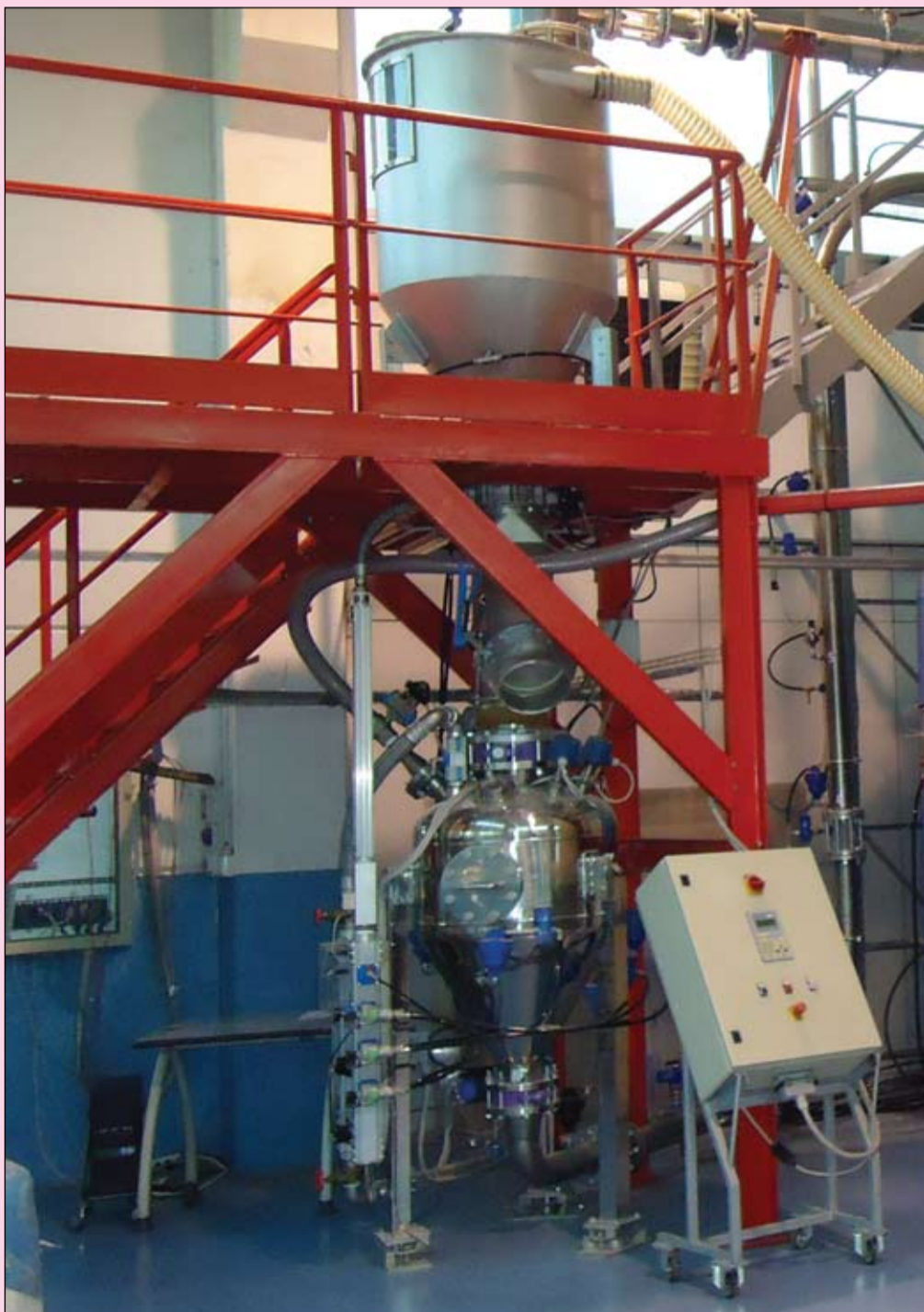
The Air-Tec system test plant at Calderara di Reno, near Bologna, offers comprehensive facilities for conducting dense phase pneumatic conveying trials.
